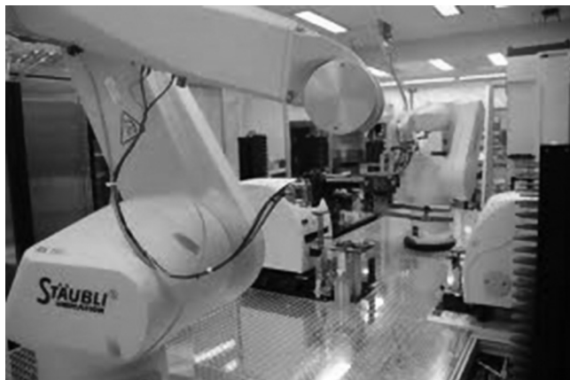
FIGURE 20.2 A large-scale robotic screening system in use at the NIH Chemical Genomics Center. This is capable of screening up to 100,000 compounds at a time. Inside the enclosure is a large robot arm that moves plates between stations.
